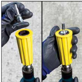
3. Insert and Lock in X-PRESS Anchor
