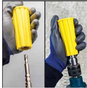
2. Attach X-PRESS It™ 2.0 Sleeve
