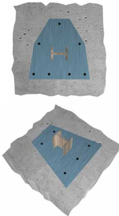
Customize base plate shapes and anchor layouts
